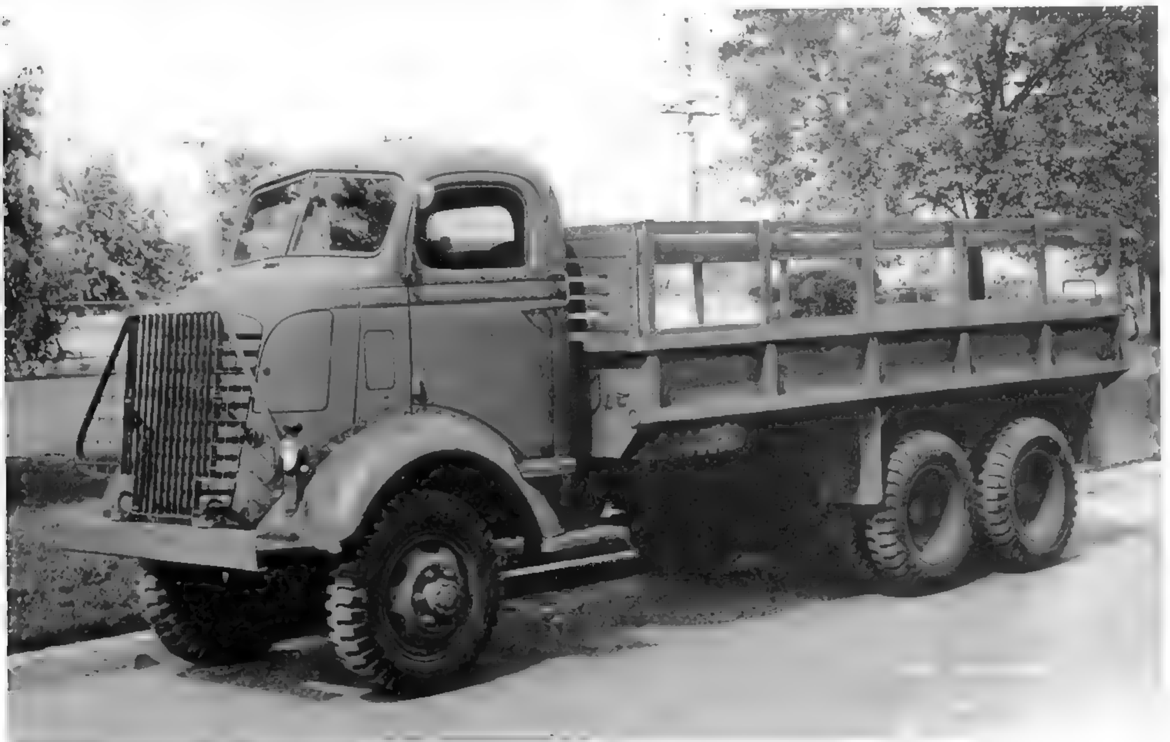
This is the AFKWX-353 in its earliest form, with a closed cab and 15-ft. steel cargo bed. (Photo from Bryce Sunderlin collection)
